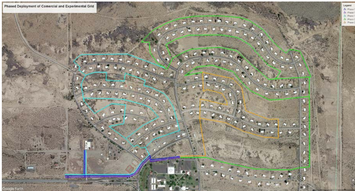
Figure 2: The combined experimental power grid and new commercial power grid will be installed in a phased approach utilizing the same trenches as the fiber optic cable layout; Blue elements are in the first phase, green elements are in the second phase and orange elements are in the third phase
