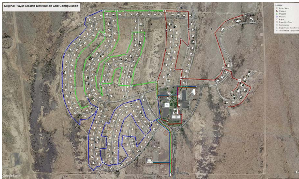
Figure 4: Original power grid configuration showing three phases of distribution system
