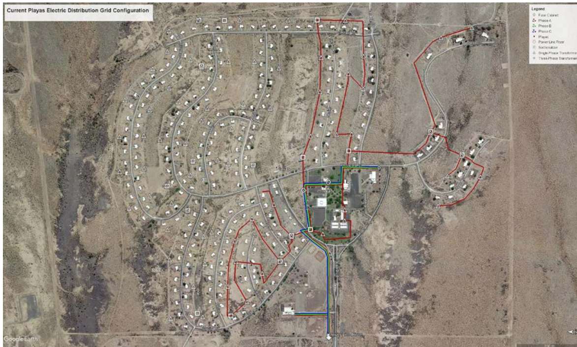
Figure 5: Current configuration of the power grid showing only a single phase is operational in a portion of the facility
