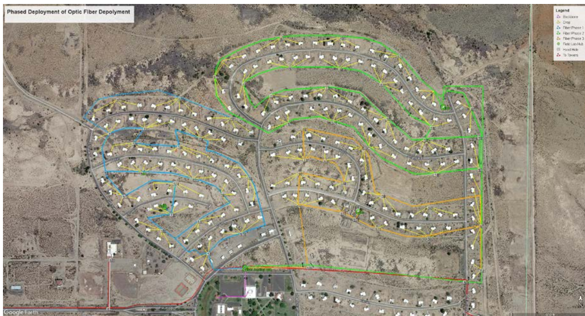
Figure 6: The phased approach for fiber layout will be done in tandem with the phased installation of power; blue and red elements will be installed in the first phase, green elements in the second phase, and orange in the third phase; not pictured is the line to the airstrip
