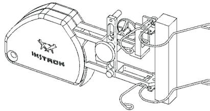
Figure 3-4. Wire clips in use
