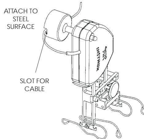
*Figure 3-10. Extensometer suspended from cleat post — steel covered machines*
