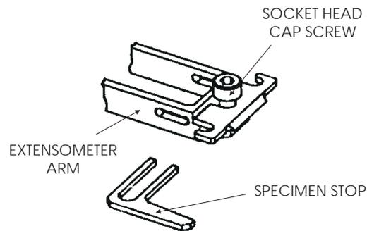
*Figure 3-12. Specimen Stops*
