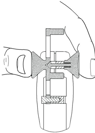
*Figure 3-2. Gauge Length Setting
