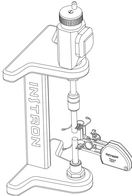
*Figure 3-13. Extensometer mounted on an optional calibration fixture (Cat. No. 2602-017)*
