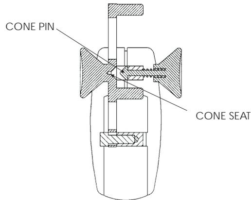
*Figure 3-1. Gauge Length Setting
