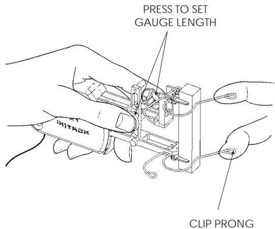
Figure 3-7. Two-handed Installation
