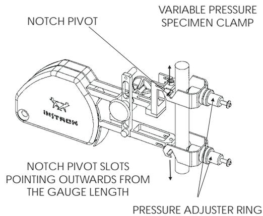
Figure 3-5. Specimen attachment using the optional Specimen Clamps and Pivot Knife Edges
