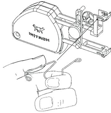
Figure 3-3. Insertion of Clips
