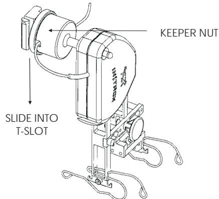
Figure 3-9. Extensometer suspended from cleat post — T-slot machines
