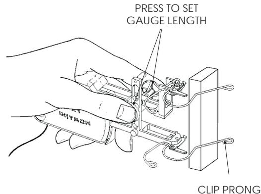
Figure 3-8. Single-handed Installation
