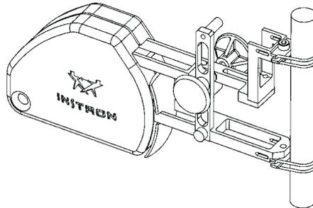
*Figure 3-6. Specimen attachment using elastic bands*
