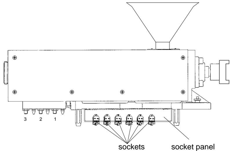
A socket panel on the right side of the extruder is provided for connecting a die with several heating connections.
