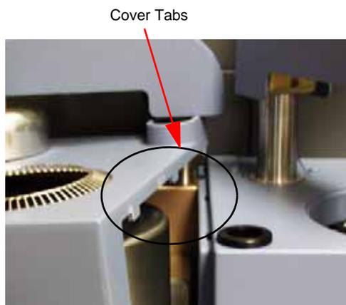
If you do not have an Autosampler, you will have to remove additional screws to release the cover. Then pull the cover towards you to remove it fully.
