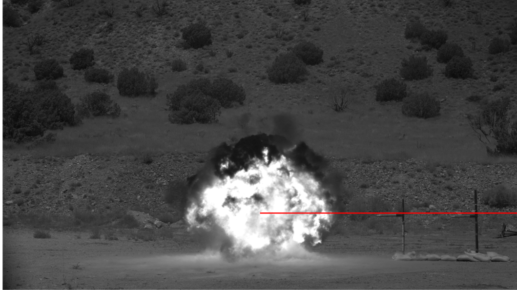
Figure 4.11: The flow-on image 10 ms after detonation. The red line depicts the row that is analyzed and ultimately converted to pressure. The line falls just above both pressure gauges, but below the triple point with the mach stem.
