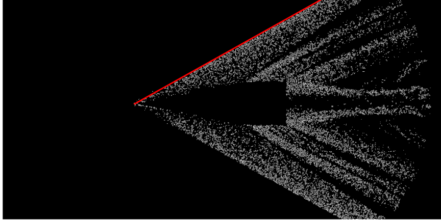
Figure 3.6: Background subtracted image with the found shock edge shown in red.
