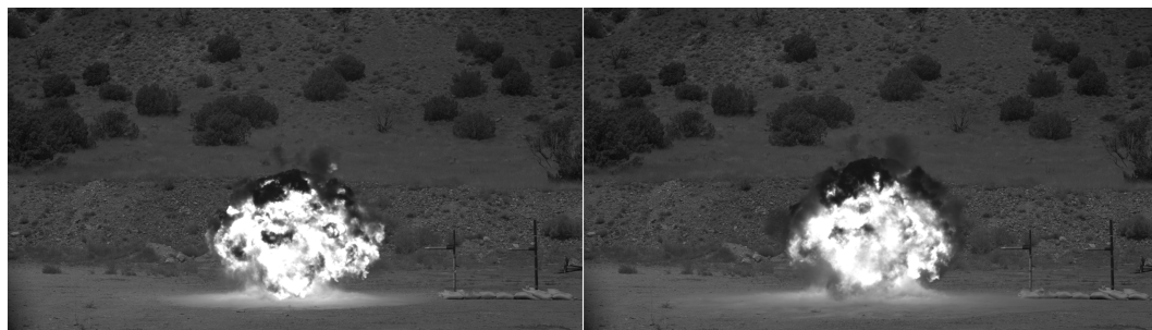
Figure 4.25: The new flow-off and flow-on image to reconstruct sequential OF. The flow-off image is 4.4 ms after detonation, and the flow-on image is 10 ms after detonation.
