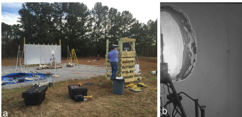
The HUCTA is positioned between the camera and screen, approximately 5 m from the screen and 15 m from the camera. A high-speed digital video camera is used to record the shadowgraph images. Figure 2 shows an image of the shadowgraph setup and a typical shadowgram from testing.
