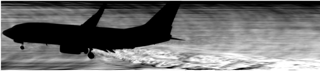
**Figure 7.** Takeoff of a 737 jetliner as visualized by Synthetic Limb Edge Schlieren (SLES). Reproduced with permission from Spectabit Optics LLC.
