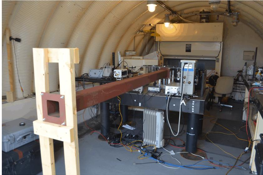
Figure 3.1: Image of the installed THOR facility in the East Lab test chamber. Centered is THOR with the open exit section facing outward. Right side is the transmitting optics. Left side beyond THOR are the receiving optics.
