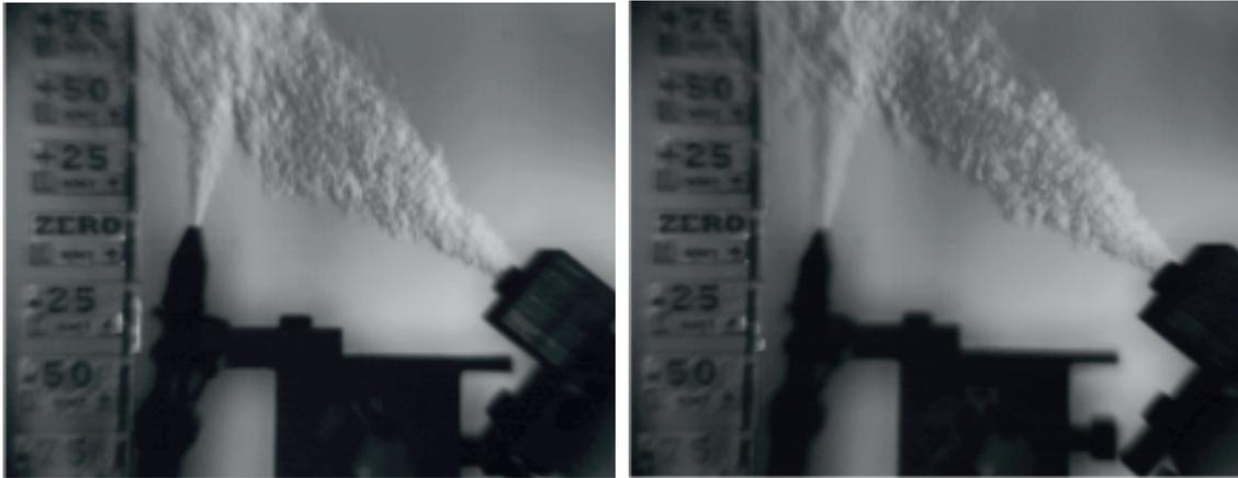
Figure 7.13: A) Crossed helium jets separated by 50 mm on the optical axis, B) Crossed helium jets separated by 300 mm on the optical axis
