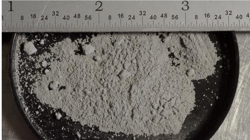
Figure 6.1:  $Al-I_2O_5$  thermite powder used for testing.
