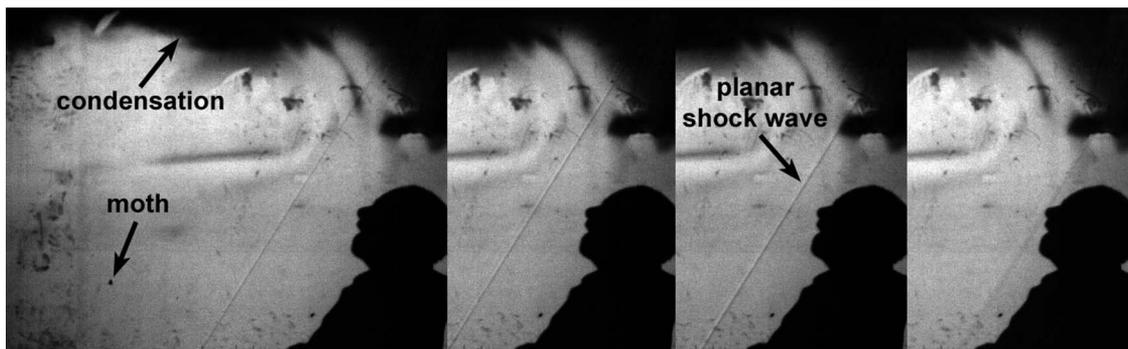
Fig. 8. Image sequence of planar shock wave propagation from a fireworks display, impinging on the author (GSS). The shock appears defocused in the leftmost and rightmost images, while it is sharp in the center two images, due to its alignment with the diverging light rays of the shadowgraph illumination.
