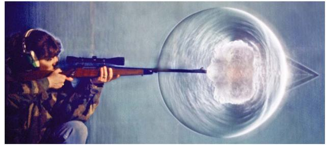
Fig. 11. (Color online) Schlieren image of the firing of a Remington .30–06 high-powered rifle using the Penn State full-scale schlieren system.
