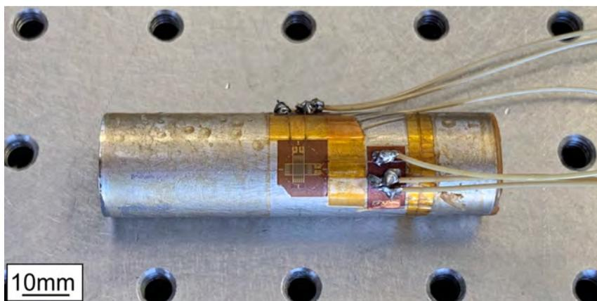
Figure 2.6: Open 18650 size battery case with strain gauge and data acquisition wiring attached.
