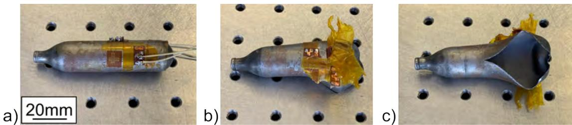
Figure 2.11: Carbon dioxide cartridge with strain gauge mounted (a) before testing and (b-c) after burst from two perspectives.
