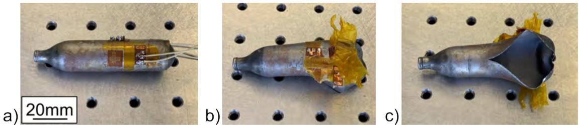
Figure 2.11: Carbon dioxide cartridge with strain gauge mounted (a) before testing and (b-c) after burst from two perspectives.
