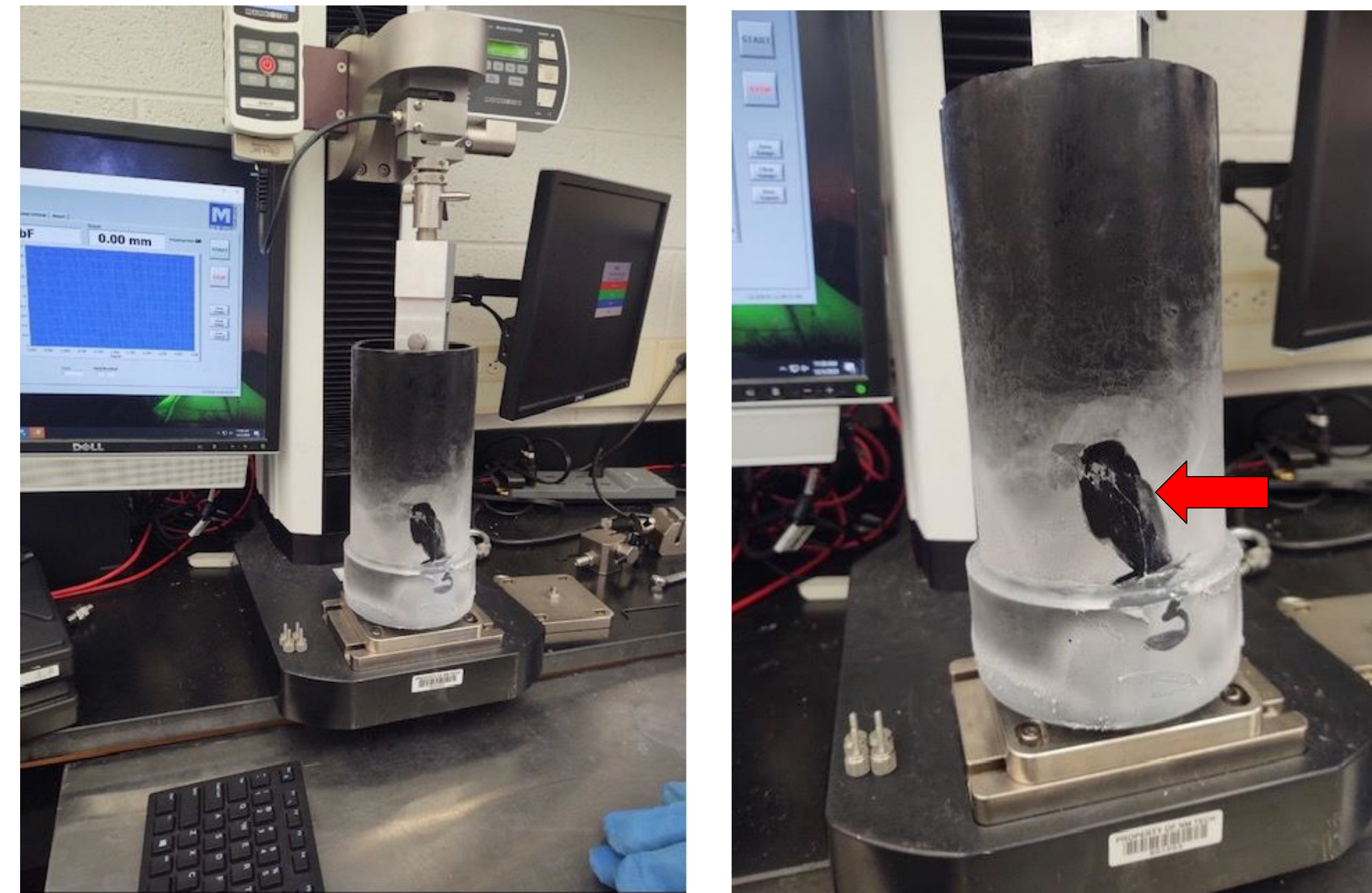
Figure 2: The original Cryogenic Bath with the exposed crack
