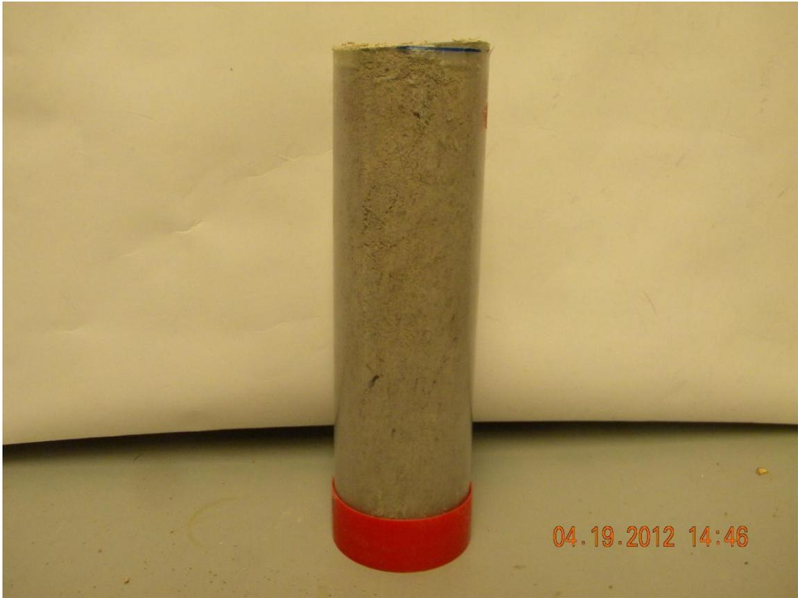
Figure 8: Representative core sample of Qct from borehole LADP-5.
