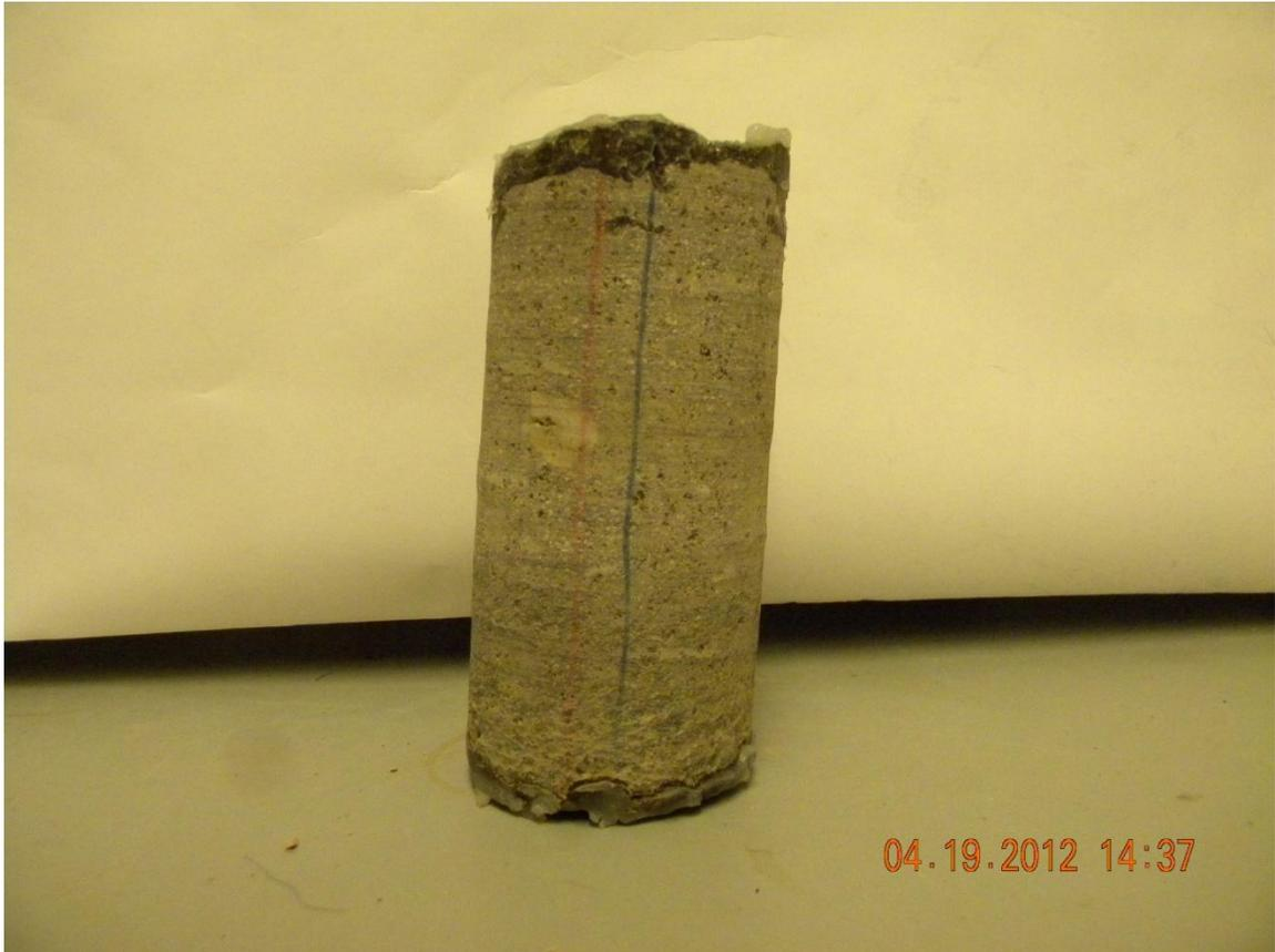
Figure 5: Representative core sample of Qbt 2 from borehole LADP-5.
