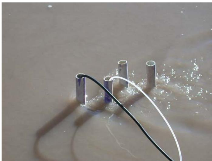
Figure 2. Picture of piezometers (leftmost, with black hose, is used for injection, others are used for sampling).
