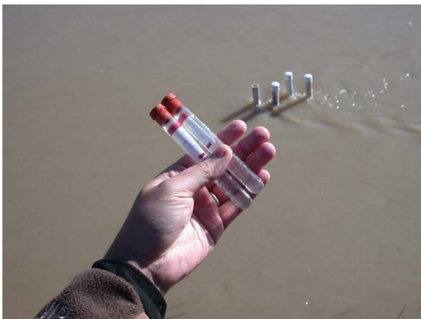
A 3-day tracer experiment (from 12/9/03 to 12/11/03) was conducted in the Rio Grande streambed along the Escondida Bridge just north of Socorro, NM. Sulfur hexafluoride (SF<sub>6</sub>), an inert, nonflammable, odorless, colorless and environmentally benign gas, was injected into the streambed in order to determine seepage fluxes and hydraulic conductivity of the sediments.
