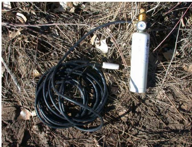
Figure 3. SF<sub>6</sub> bottle, valves, gauges, regulators, hose and diffusing stone.
