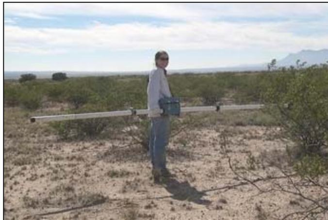
**Figure 3.2.** The EM31 meter in use, with the EM the pole being 3.7 meters long, worn at hip level in the vertical dipole position.
