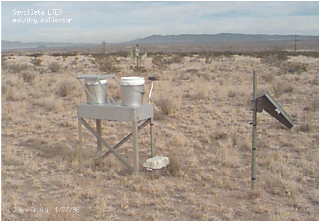
**Figure A.2.** Wet and dry chloride deposition collectors at the Río Salado Weather Station, number 44. Located above the left bucket, the wet deposition collector, is a cover that is switched to the other bucket, the dry deposition collector, during precipitation events. Picture from LTER website (Collectors 2005).
