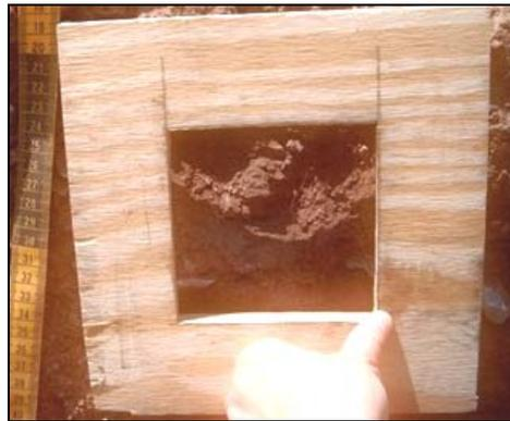
**Figure 3.5.** The 10 by 10 centimeter square used to count roots in the soil pits.
