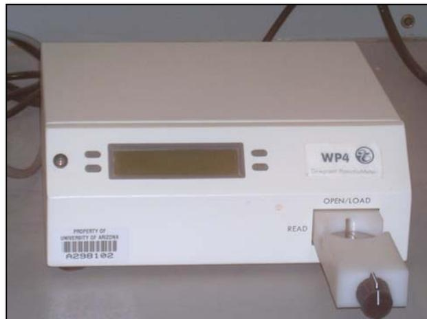
**Figure 3.4.** The water potential meter used in this study, with the sample placement drawer open.
