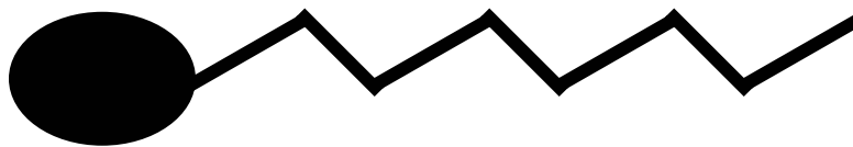
Figure 1-2. A surfactant with a long hydrophobic tail and a hydrophilic head group.
