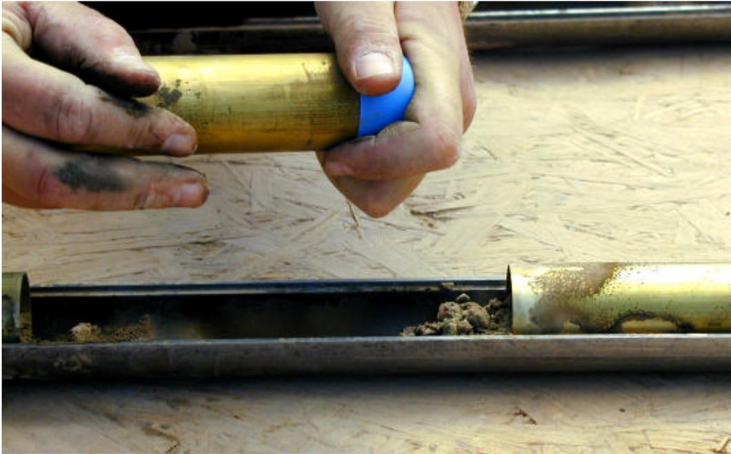
**Figure 6-9.** Core sample collection in brass-sleeves lining the split spoon.
