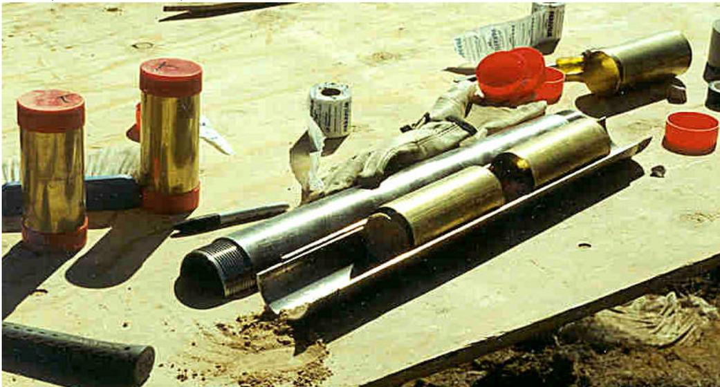
**Figure 5-7.** Split-spoon sampler lined with brass sleeves for core collection.
