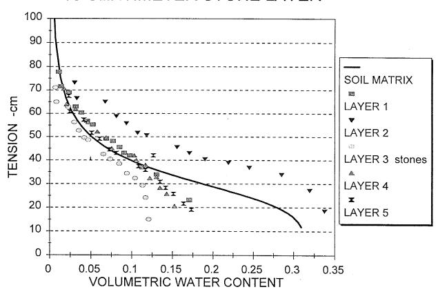
Figure 12. Soil water retention curve for the Sevilleta filed soil, heterogeneous soil profile. Impeding stone layer 10 centimeters thick in layer 3. Volumetric water content,  $(\theta_{\rm V})$ , corrected for the volume of stones present.
