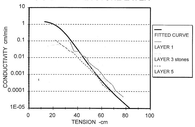
Figure 16. Unsaturated hydraulic conductivity verses tension. Heterogeneous soil profile, 10 centimeter stone layer.
