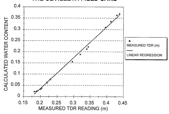
Figure 2. TDR calibration curve for the Sevilleta field sand.
