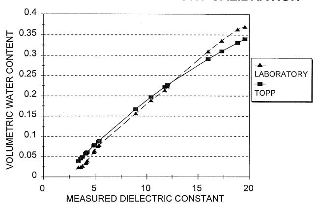
Figure A-2. Comparison of estimated volumetric water content using the equation of Topp et al. (1980) as compared to that calculated using the laboratory calibration curve determined in this study.
