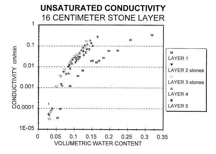
Figure 22. Unsaturated hydraulic conductivity verses volumetric water content,  $(\theta_v)$ , heterogeneous soil profile. Water content corrected for the volume of stones present.
