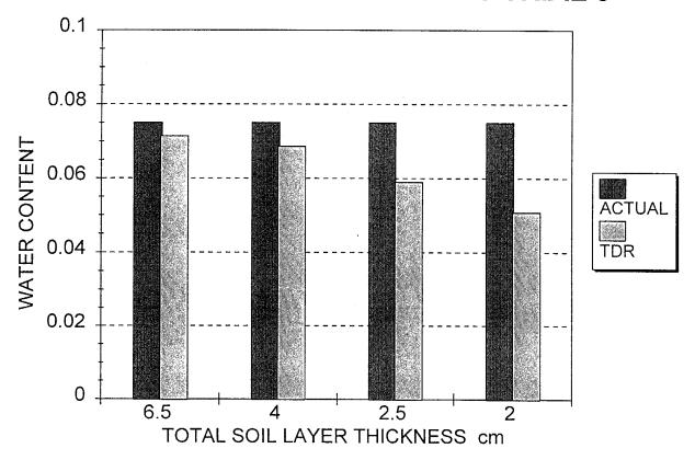
Figure 6. Influence of soil layer thickness on Time Domain Reflectometry measurement of soil water content. Trial 3, approximately eight percent water content.
