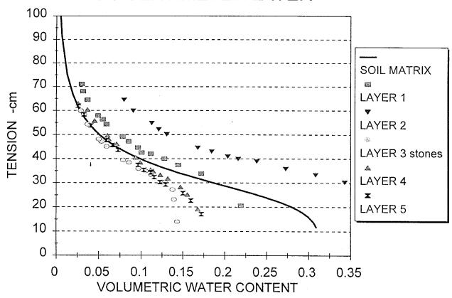
Figure 11. Soil water retention curve for the Sevilleta field soil, heterogeneous soil profile. Impeding stone layer 6.5 centimeters thick in layer three. Volumetric water content,  $(\theta_v)$ , corrected for the volume of stones present.
