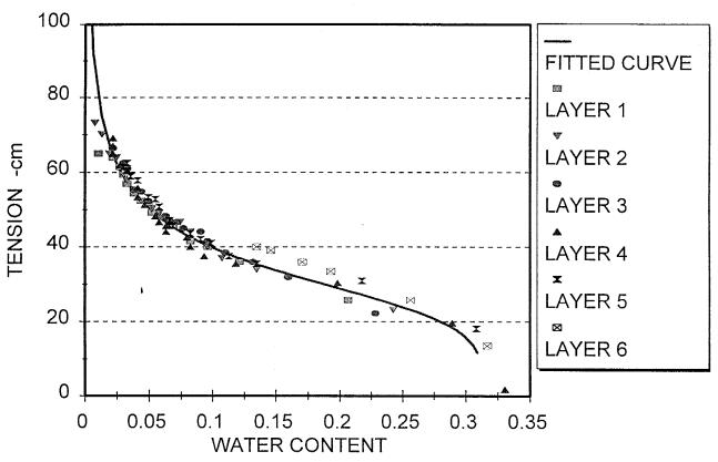
Figure 10. Soil water retention curve for the Sevilleta field soil, homogeneous soil profile. RETC curve fit utilizing the models of van Genuchten and Mualem.
