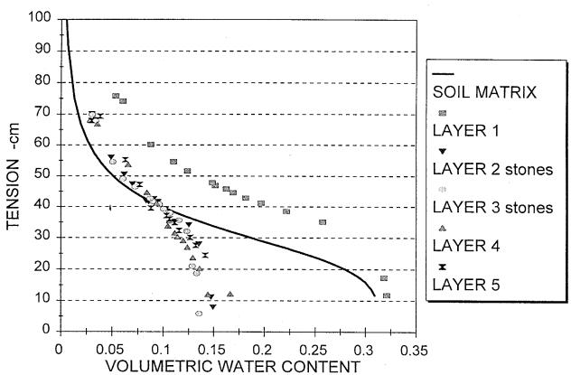
Figure 13. Soil water retention curve for the Sevilleta field soil, heterogeneous soil profile. Impeding stone layer 16 centimeters thick in layers two and three. Volumetric water content,  $(\theta_{v})$ , corrected for the volume of stones present.
