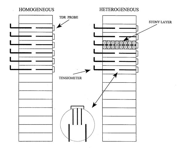
Figure 1. Schematic representation of soil columns illustrating homogeneous and heterogeneous profiles, along with instrument placement.
