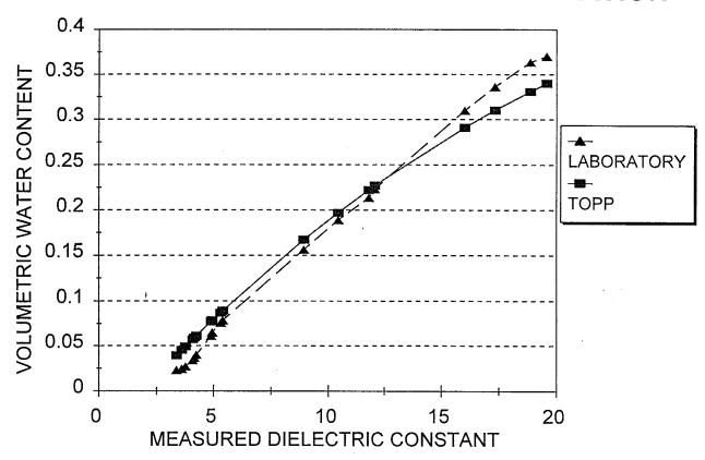
Figure 3. Comparison of estimated volumetric water content using the equation of Topp et al. (1980) as compared to that calculated using the laboratory calibration curve determined in this study.
