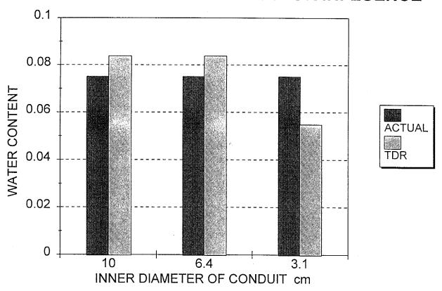
Figure 8. Sensitivity of Time Domain Reflectometry measurements to the removal of outer wave guide contribution.
