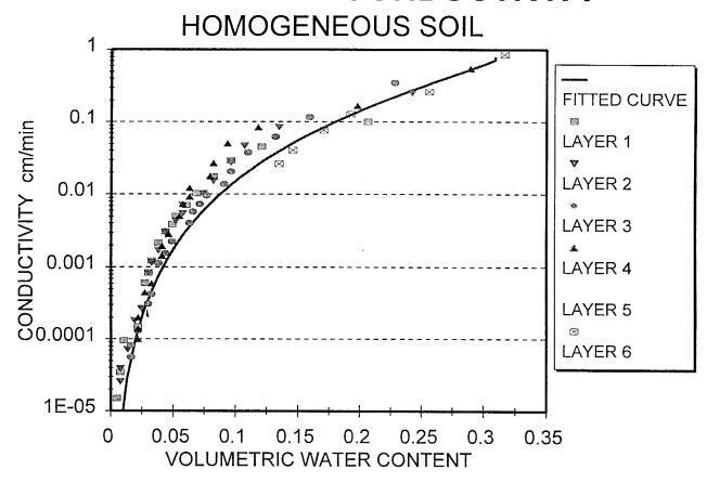
Figure 18. Unsaturated hydraulic conductivity verses volumetric water content, homogeneous soil profile. RETC curve fit utilizing the models of van Genuchten and Mualem.
