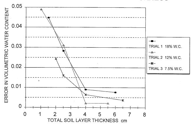
Figure 7. The observed error in volumetric water content between calculated and measured water content, as a function of soil layer thickness, for three soils having different initial water contents.
