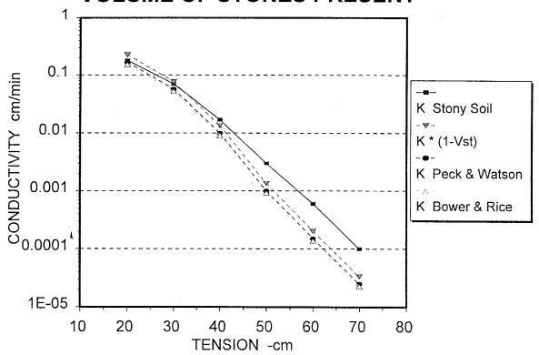
Figure 23. Correction of conductivity for the volume of stones present in the soil profile, conductivity verses tension for the 10 centimeter stone layer. A comparison of various methods.
