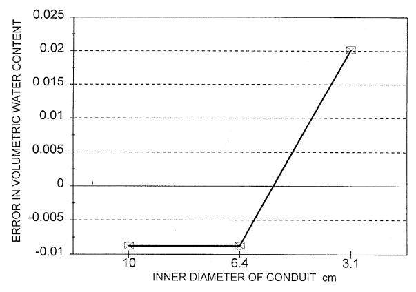
Figure 9. Error in the Time Domain Reflectometry measurement of a moist soil, removal of outer conductor contribution to the reading.
