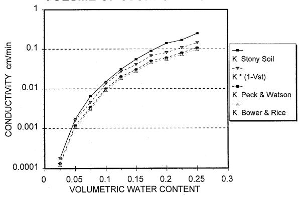
Figure 24. Correction of conductivity for the volume of stones present in the soil profile, conductivity verses volumetric water content for the 10 centimeter stone layer. A comparison of various methods.
