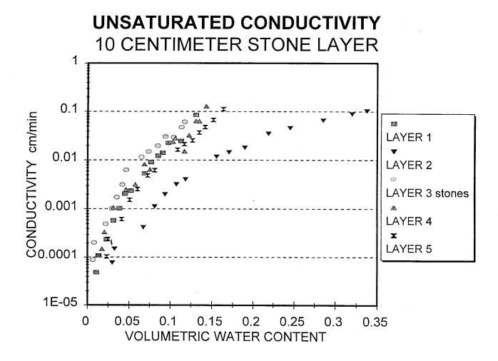
Figure 21. Unsaturated hydraulic conductivity verses volumetric water content,  $(\theta_v)$ , heterogeneous soil profile. Water content corrected for the volume of stones present.
