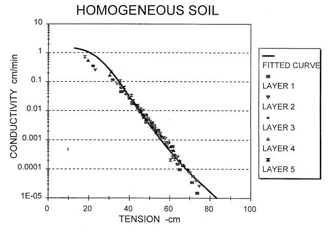
Figure 14. Unsaturated hydraulic conductivity verses tension, homogeneous soil profile. RETC fitted curve utilizing the models of *van Genuchten* and *Mualem*.
