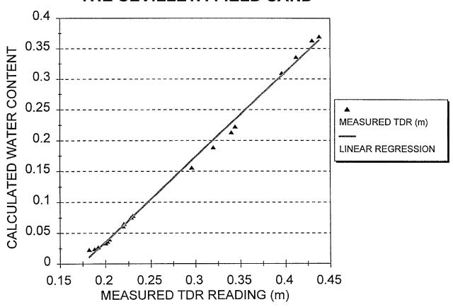
Figure A-1. TDR calibration curve for the Sevilleta field sand.
