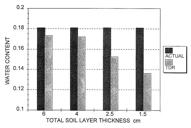
Figure 4. Influence of soil layer thickness on Time Domain Reflectometry measurement of soil water content. Trial 1, approximately eighteen percent water content.
