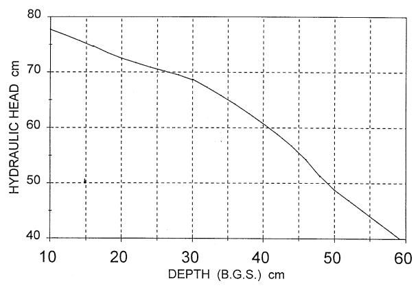
Figure 20. Computer simulation of the head with depth profile for a heterogeneous soil column using Chain \_2D.
