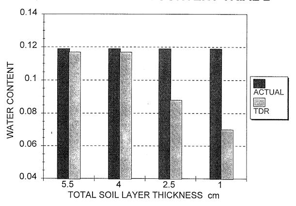
Figure 5. Influence of soil layer thickness on Time Domain Reflectometry measurement of soil water content. Trial 2, approximately twelve percent water content.
