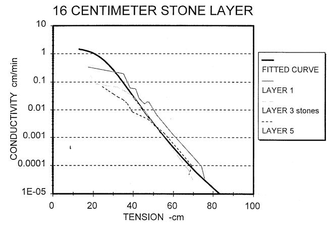
Figure 17. Unsaturated hydraulic conductivity verses tension. Heterogeneous soil profile, 16 centimeter stone layer.
