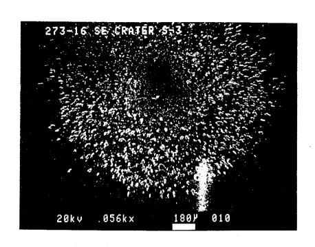
Figure 21. Nickel and Silver Secondary Reactions.
