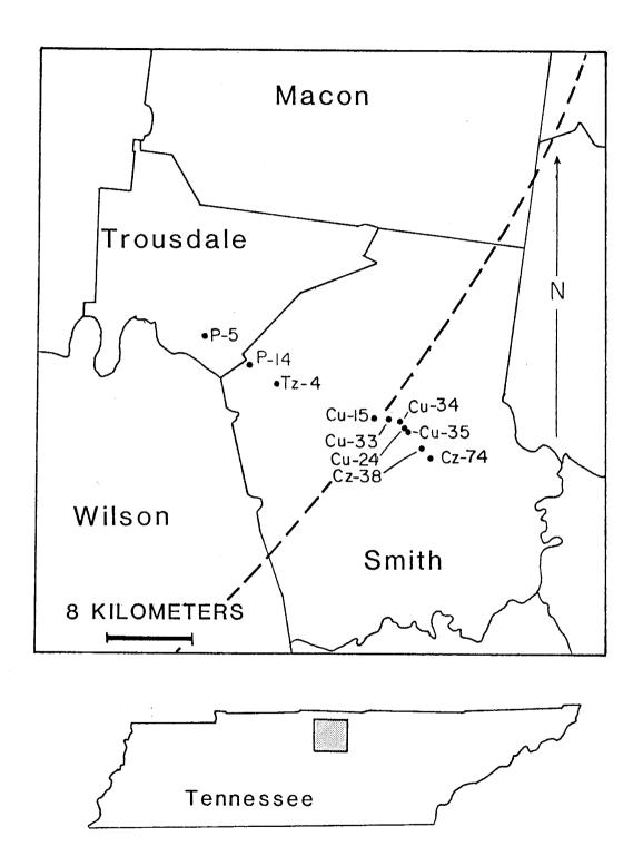
Mineralization in the district is scattered laterally and stratigraphically in the karstified, Lower Ordovician Knox Dolomite (Fig. 17). Sphalerite is the only mineral mined in the district. Fluorite, barite, calcite, dolomite, and galena are also present (Kyle, 1973).
