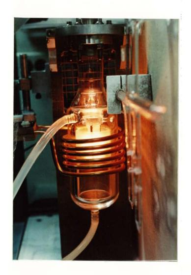
Figure 32. Argon extraction sample bottle.
