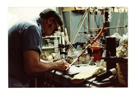
Figure 30. Closure of an irradiation vial. The quartz glass vials are heat sealed under a low vacuum. Pictured is scientific glassblower Alfred Heine of Virginia.
