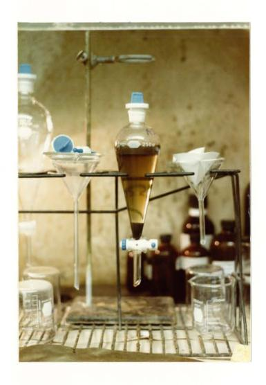
Figure 27. Heavy liquid mineral separation, showing the separation of a sample due to density differences between the minerals.
