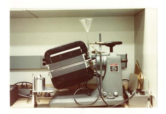
Figure 26. Frantz isodynamic magnetic separator, featuring a modified sample feed system, located in the U. S. Geological Survey, Reston, Virginia.
