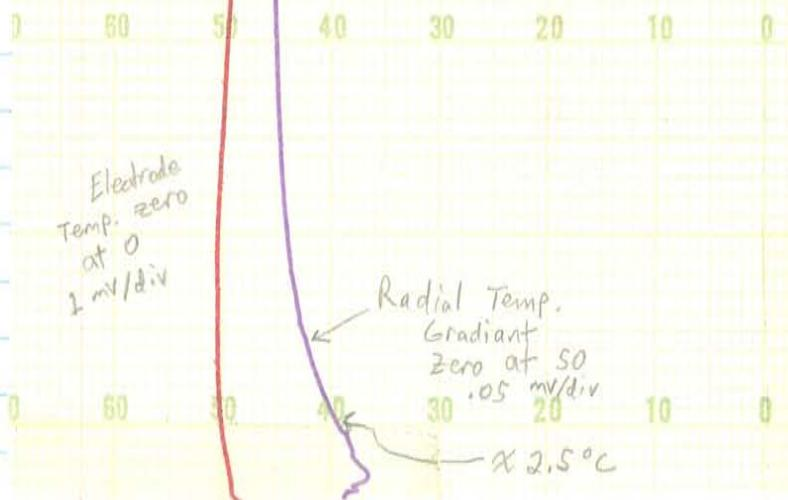
Ice sample is  $\approx \frac{1}{2}$ " thick. It was cooled rapidly and then allowed to sit for  $\approx 2$  minutes. Temp. was controlled at  $-100^\circ\text{C}$  before cooling
