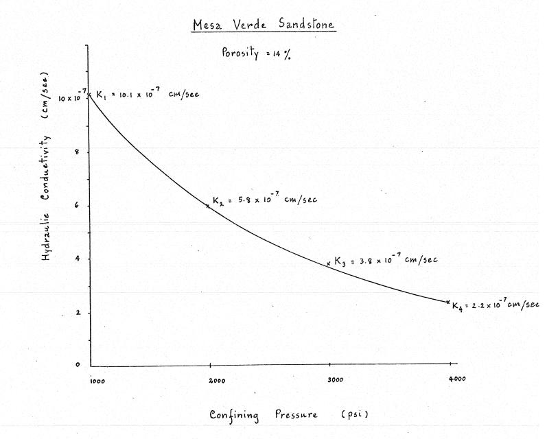
Fig. 5 Hydraulic conductivity vs. confining pressure on Point Lockout Sandstone.
