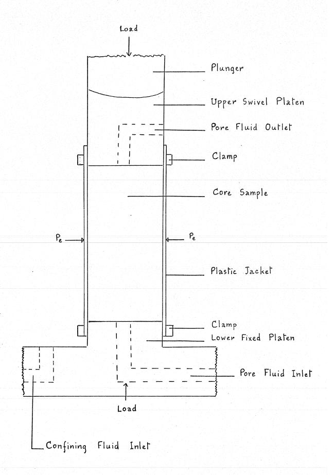
Fig. 2 Diagramatic sketch of experimental equipment.
