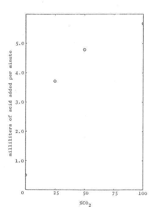
Figure 6. Plot of the dissolution rate of strontianite, calculated using equation (48), versus  $P_{\rm CO_2}$  for strontianite dissolution at 40° C and pH = 4.5.
