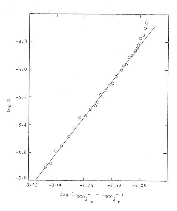
Figure 27. Plot of  $\log (m_{HCO_3} - m_{HCO_3})$  wersus time in minutes for strontianite dissolution at 40°C and  $P_{CO_2} = 0.81$  atmosphere. The slope of the line, 2.29 x 10<sup>-3</sup>, is essentially the same as that determined using  $\log (m_{Sr}^2 + m_{Sr}^2 + m_{Sr}^2$
