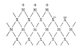
where a residual positive charge, +, is associated with the lattice cation, M, and a residual negative charge, -, is associated with the lattice anion group, X. For experiments run under a nitrogen atmosphere, the value of  $(m_{Me}^{2+})$  is infinite with respect to strontianite saturation if  $(m_{Me}^{2+})$  is removed from the system. Therefore, the rate limiting step is interpreted to be the interaction of a hydrogen ion at an anion position on the surface.
