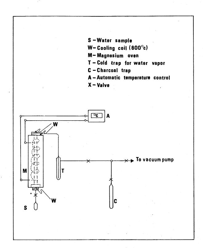
Fig. 4 Details of conversion system
