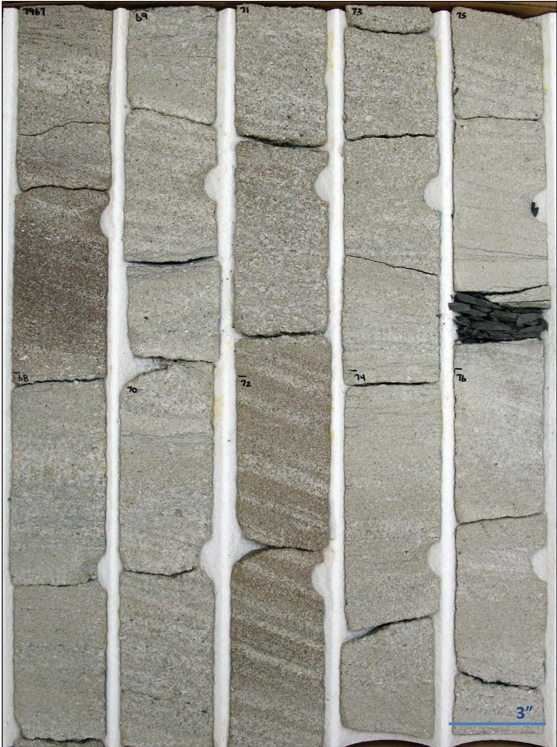
**Figure 16.** Well 32-6, 7967 ft to 7977 ft. In well 32-6, the Coarse-grained Sandstone facies exhibits considerable variation in grain size at the centimeter scale, alternating in size between coarse sand and conglomerate. Note hematite staining, clay seams, and mudstone interbed.
