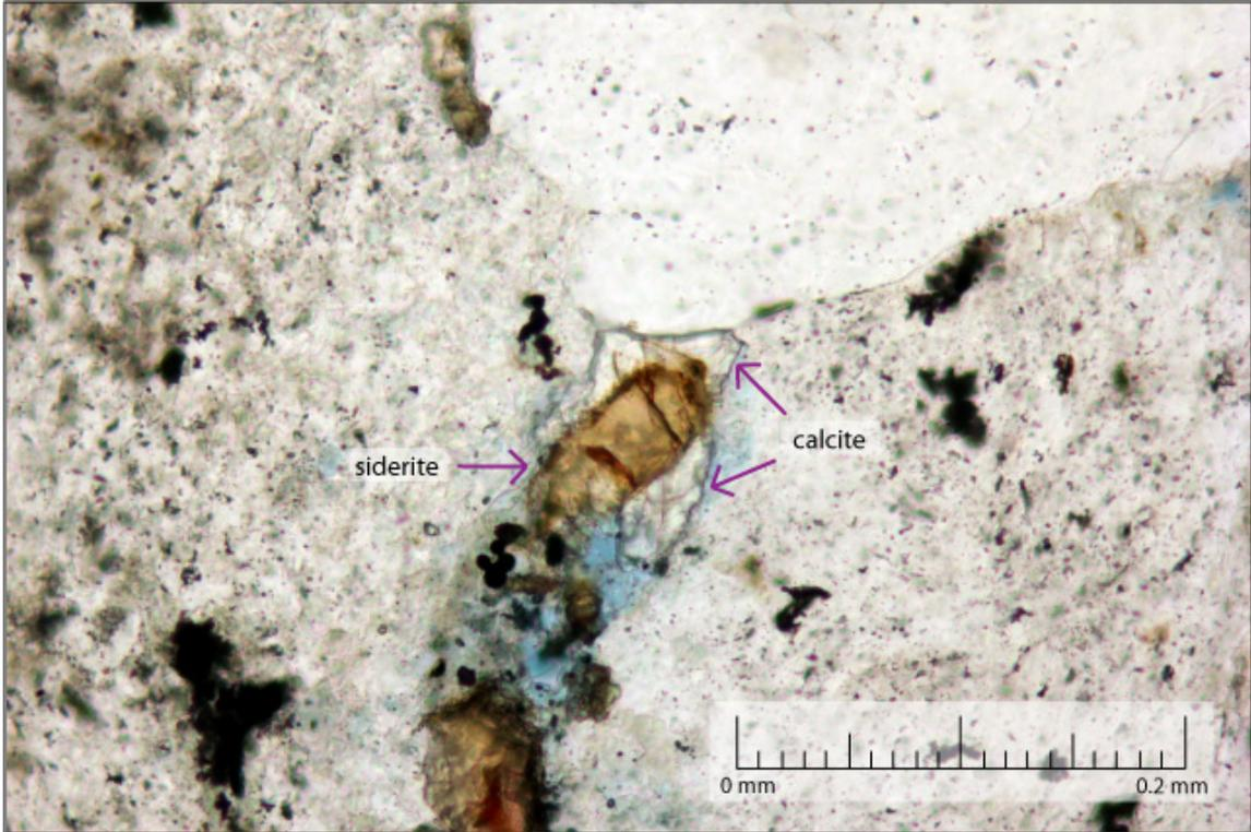
**Figure 44.** Well 42-1, 8015.5 ft, ppl. Calcite precipitated on a siderite crystal, indicating that siderite precipitated before the calcite.
