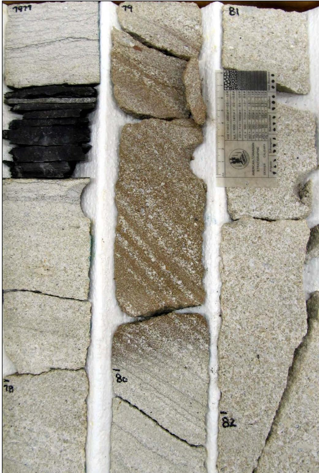
**Figure 20.** Well 32-6, 7977 ft to 7782 ft. Coarse-grained Sandstone facies. Hematite stained, over-steepened cross beds exhibiting possible rhythmite sets. Note mudstone interbed in upper left corner. This bed contained very small shell fragments.
