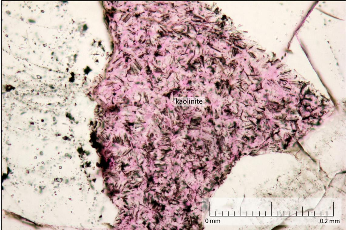
**Figure 62.** Well 13-10A, 7675.90 ft. This oil-stained kaolinite indicates that oil emplacement occurred after the precipitation of kaolinite. This kaolinite also displays authigenic textures in the form of delicate booklets.
