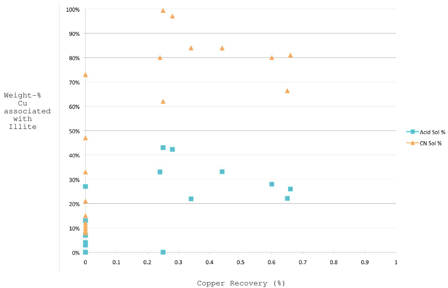
**Figure 19:** Weight percentage of copper associated with illite versus copper recovery. No correlation was identified that as total copper values increases so does copper recovery.
