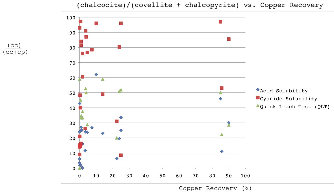
**Figure 11:** Scattergram illustrating chalcocite (cc) / covellite (cv) + chalcopyrite (cp) verses the three copper solubility tests used in this study. Generally speaking, there is no correlation between increasing sulfide ratios and recovery values. This lack of correlation is because copper is present in other copper-bearing mineral phases such as goethite, copper-bearing clays, and encapsulated copper sulfides, which are not considered during the line integration ratios.
