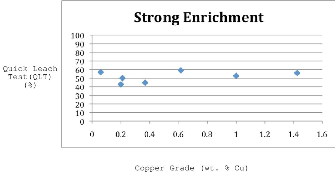
**Figure 31:** Quick Leach Test (QLT) solubility versus copper grade representing data values from strong enrichment. As the copper grade increases the leachability is constant.
