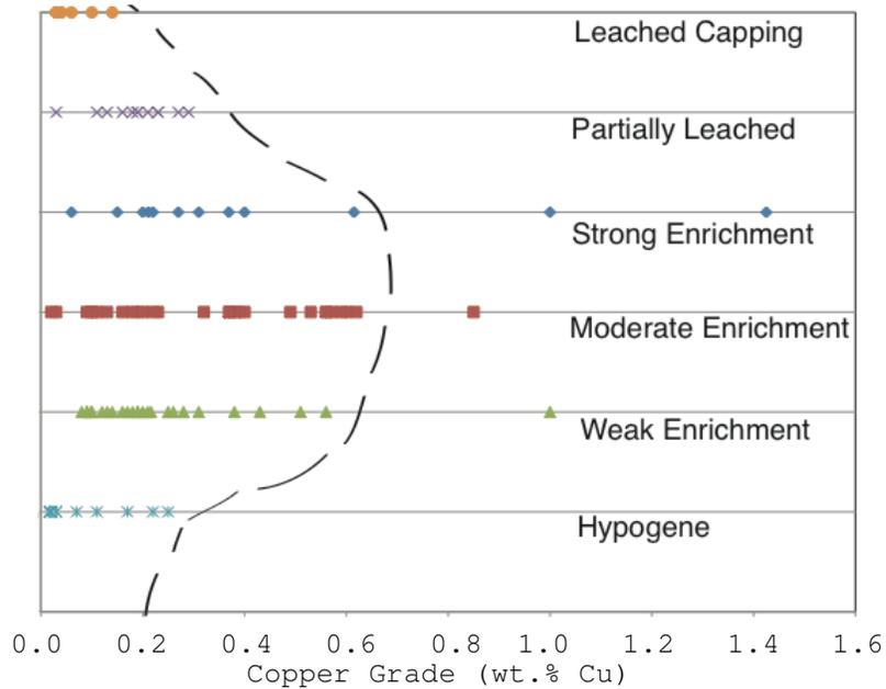
**Figure 13:** Graphical geochemical zonation representing the varying copper grade with respect to copper ore type. Copper grade increases at the Strong Enrichment zone and then diminishes with depth approaching the hypogene zone. Note protore average grade is 0.14% Cu with an approximate enrichment factor of 0.71.
