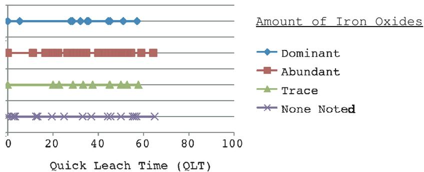
**Figure 34:** Line graph illustrating the abundances of iron oxides in correlation to Quick Leach Time (QLT). The overlapping values indicate that the amount of iron oxides does not influence QLT. Dominant (n=19), Abundant (n=45), Trace (n=13), and none noted (n=21).
