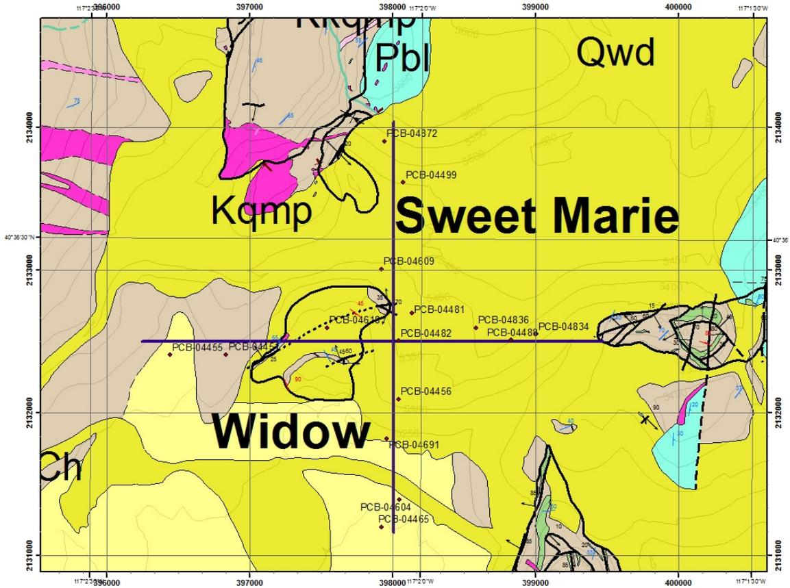
**Figure 5:** Generalized geologic mp of the Widow Pit showing the location of cross-section modified from Keeler, 2010.
