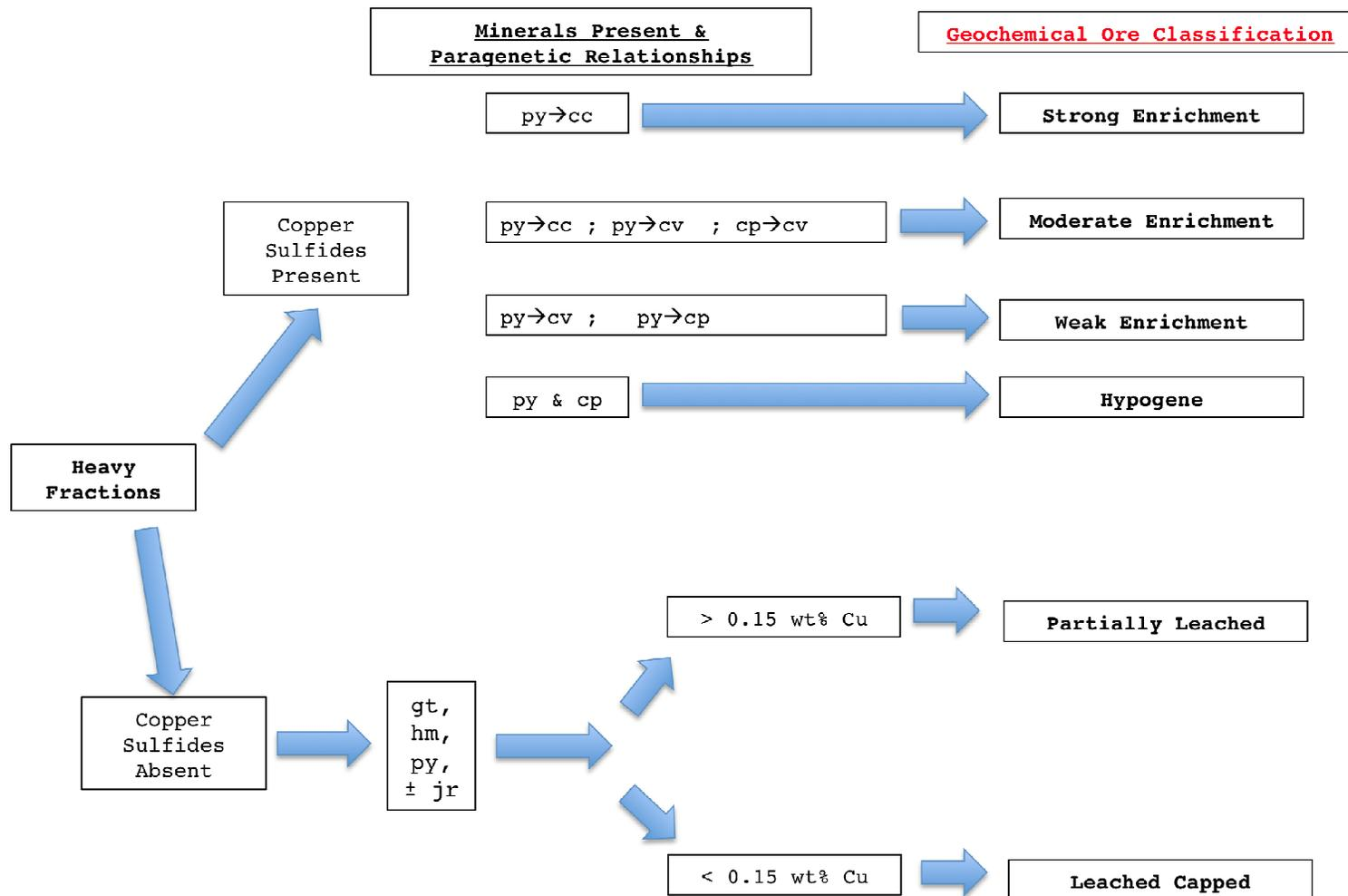
**Figure 6:** Flowchart of geochemical logging used in the petrographic analysis for the current study. (cc) chalcocite, (cp) chalcopyrite, (cv) covellite, (gt) goethite, (hm) hematite, (jr) jarosite, (py) pyrite, and ( → ) replaced by
