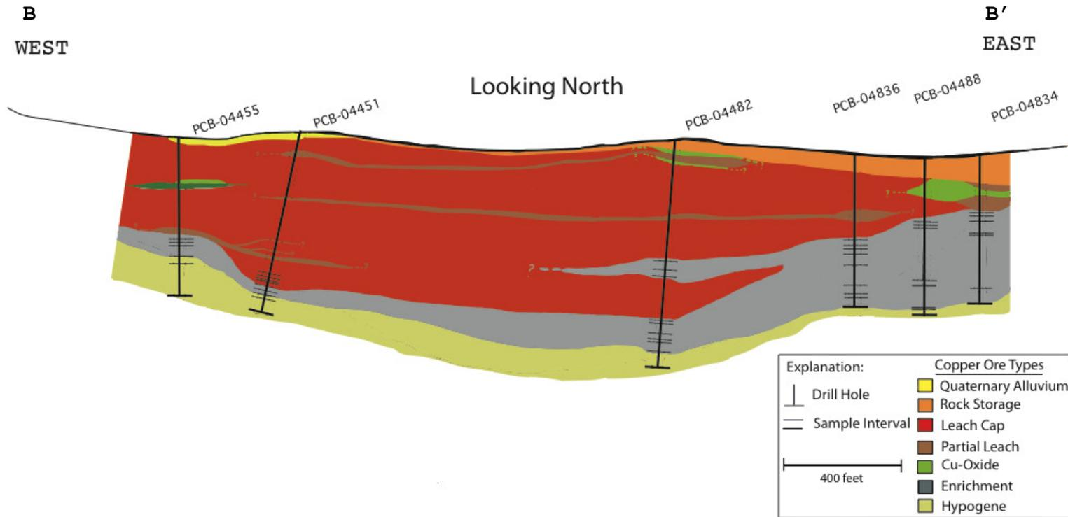
**Figure 36:** West-East cross section illustrating the mineralogy and geochemistry of the supergene enrichment profile of the Widow Pit, Copper Basin, Nevada
