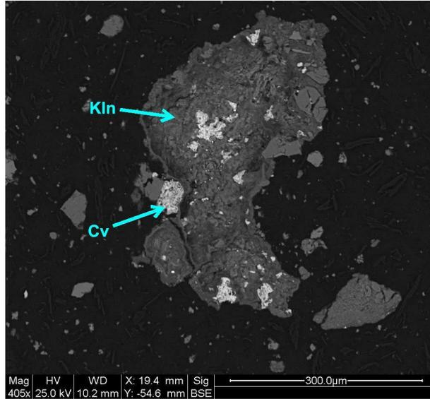
**Figure 16:** Backscatter electron image of covellite (bright minerals labeled Cv) within a kaolinite (Kln) particle of a sample from around the Widow Pit indicating copper sulfide encapsulation (Thogerson, 2012).
