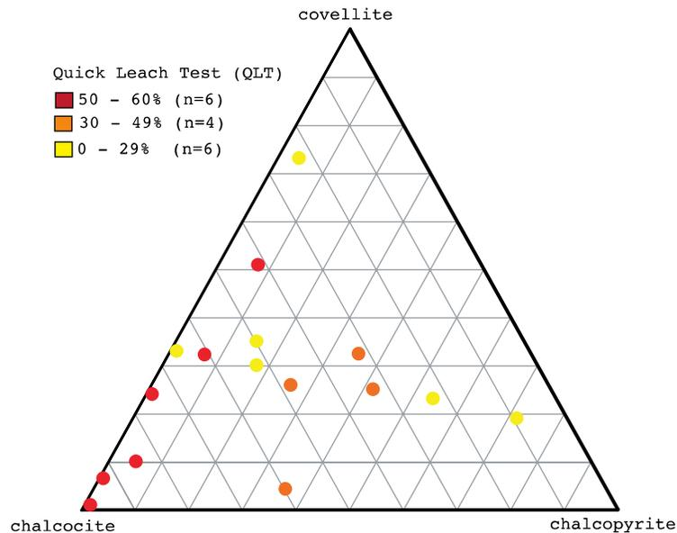
**Figure 30:** Ternary diagram illustrating copper sulfide composition corresponding to varying QLT values. This diagram shows that higher QLT values, ranging from 50 to 60% copper recovery consist of dominantly chalcocite and covellite, where as the lower QLT values ranging from 0 to 49% consist of more covellite and chalcopyrite than chalcocite. This indicates that as the amount of copper attributed to copper sulfides increases so does its leachability.
