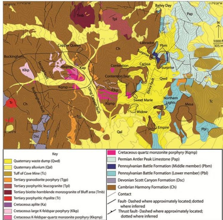
**Figure 2.** Geologic map of Copper Basin site illustrating all of the major stratigraphic rock units and structural components present within the area, Keeler, 2010 and Newmont Internal report, 2011.
