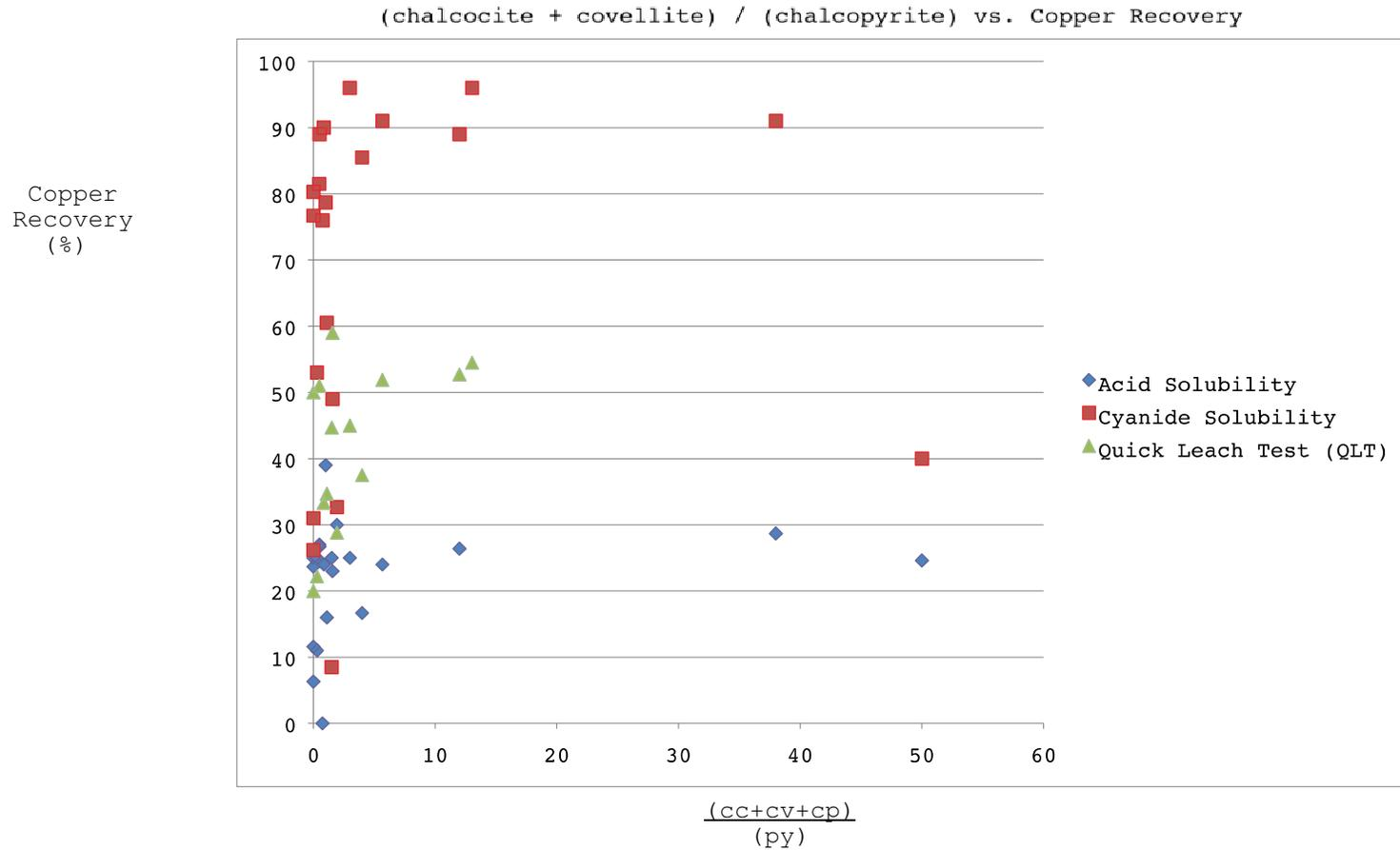
**Figure 10:** Scattergram illustrating chalcocite (cc) + covellite (cv) / chalcopyrite (cp) verses the three copper solubility tests used in this study. High ratios are associated with higher recovery values, where the lower ratios have varying recovery values. This lack of correlation is because copper is present in other copper-bearing mineral phases such as goethite, copper-bearing clays, and encapsulated copper sulfides, which are not considered during the line integration ratios.
