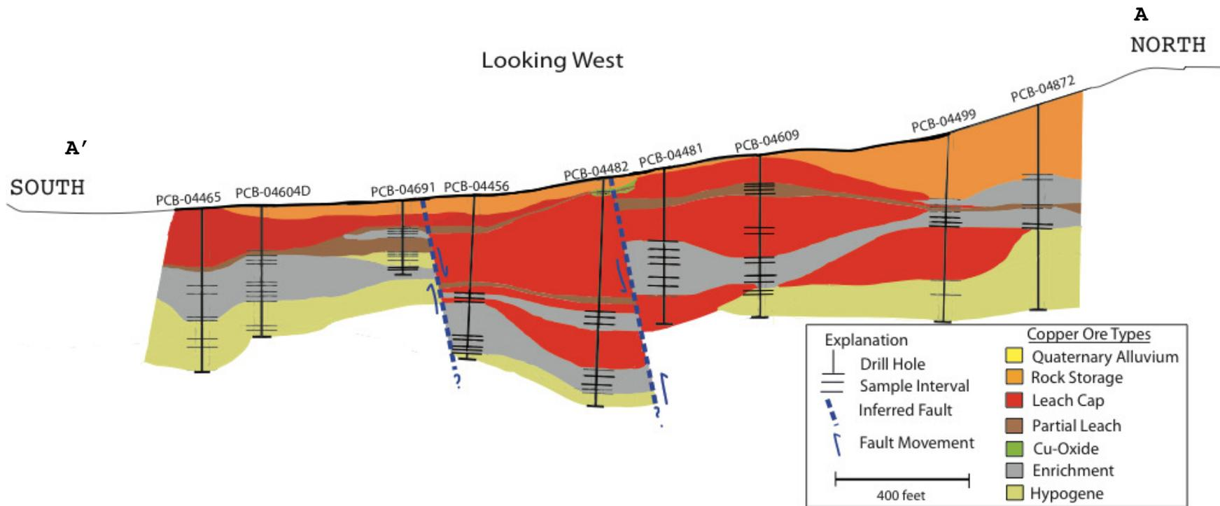
**Figure 35:** South-North cross section illustrating the mineralogy and geochemistry of the supergene enrichment profile of the Widow Pit, Copper Basin, Nevada.
