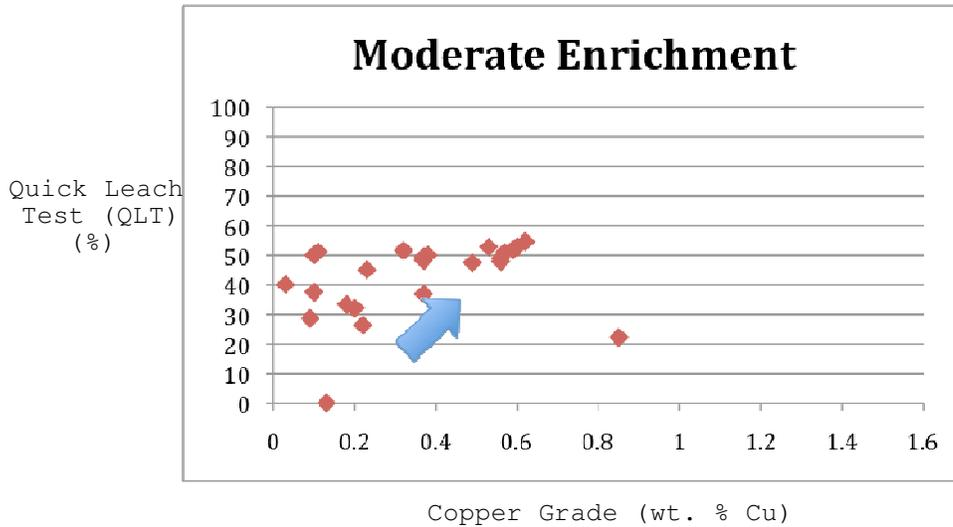
**Figure 32:** Quick Leach Test (QLT) solubility versus copper grade representing data values from moderate enrichment. As the copper grade increases so does the leachability.
