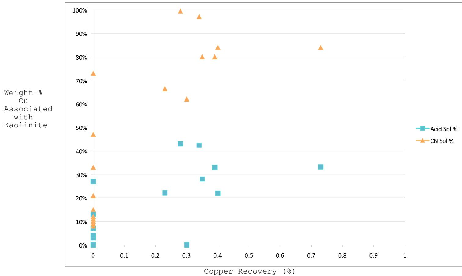
**Figure 18:** Weight percentage of copper associated with kaolinite versus copper recovery. No apparent correlation is recognized that as total copper values increases so does copper recovery.
