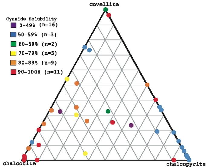
**Figure 25:** Ternary diagram illustrating the different copper sulfide composition corresponding to varying cyanide solubilities. Although there was some data clustering consisting of dominantly chalcopyrite overall, this figure indicates that copper sulfide mineralogy does not influence cyanide leachability.
