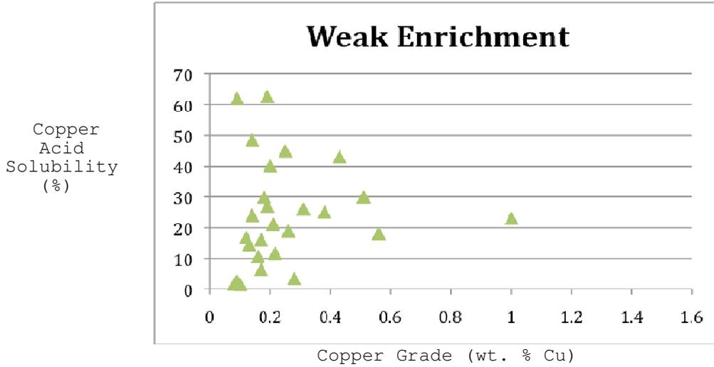
**Figure 23:** Acid solubility versus ore grade representing data values from weak enrichment. The ore grade has no influence on acid leachability, which could be due to the intermediate copper sulfide phases covellite and chalcopyrite and their varying acid solubility values, and possibly the masking by encapsulation, copper adsorbed on to goethite, and copper-bearing clays
