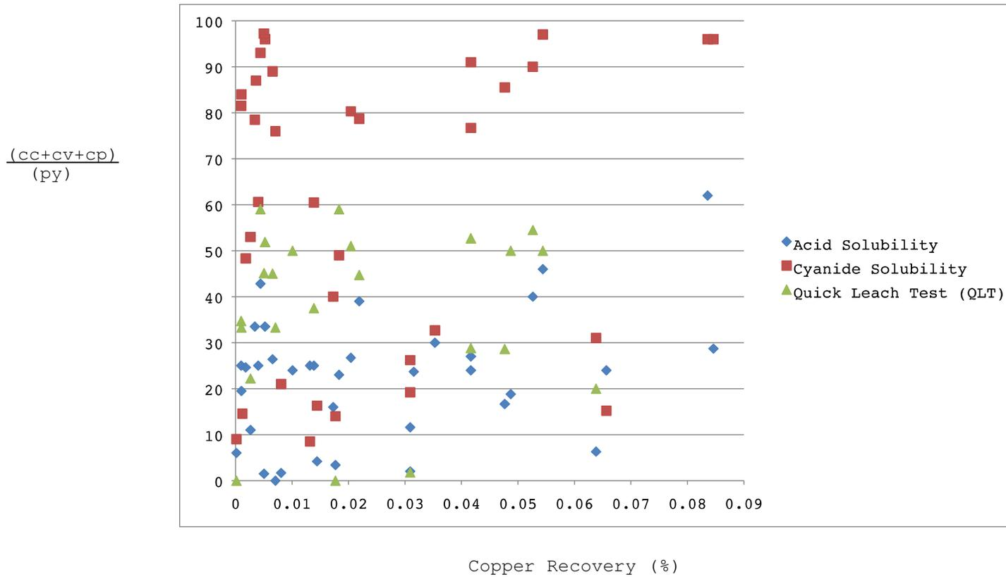
**Figure 12:** Scattergram illustrating chalcocite (cc) + covellite (cv) + chalcopyrite (cp) / pyrite (py) versus the three copper solubility tests used in this study. Generally speaking, there is no correlation between increasing sulfide ratios and recovery values. This lack of correlation is because copper is present in other copper-bearing mineral phases such as goethite, copper-bearing clays, and encapsulated copper sulfides, which are not considered during the line integration ratios.
