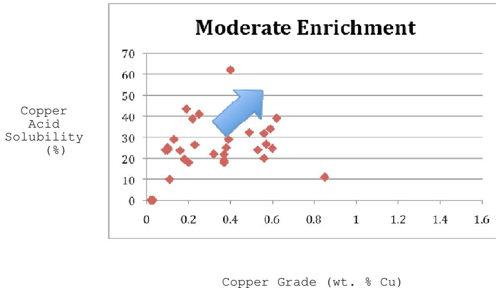
**Figure 22:** Acid solubility versus copper grade representing data values from moderate enrichment. The copper grade has no influence on acid leachability, which could be due to the intermediate copper sulfide phases covellite and chalcopyrite and their varying acid solubility values, and possibly the masking by encapsulation, copper adsorbed on to goethite, and copper-bearing clays.
