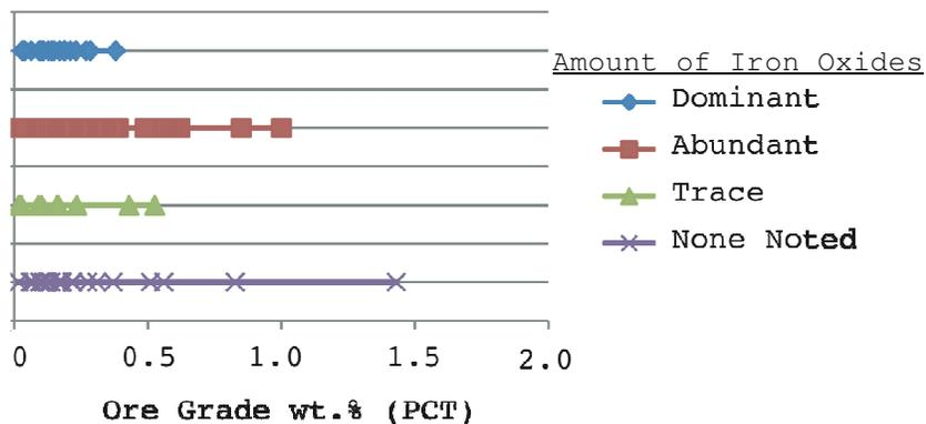
**Figure 17:** Line graph illustrating the abundances of iron oxides versus copper grade in heavy separates. It is observed that the amount of iron oxides does not influence overall copper grade. Dominant (n=19), Abundant (n=45), Trace (n=13), and none noted (n=21).
