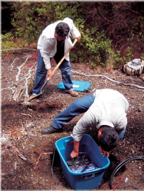
**Students digging holes and installing seismic equipment**
