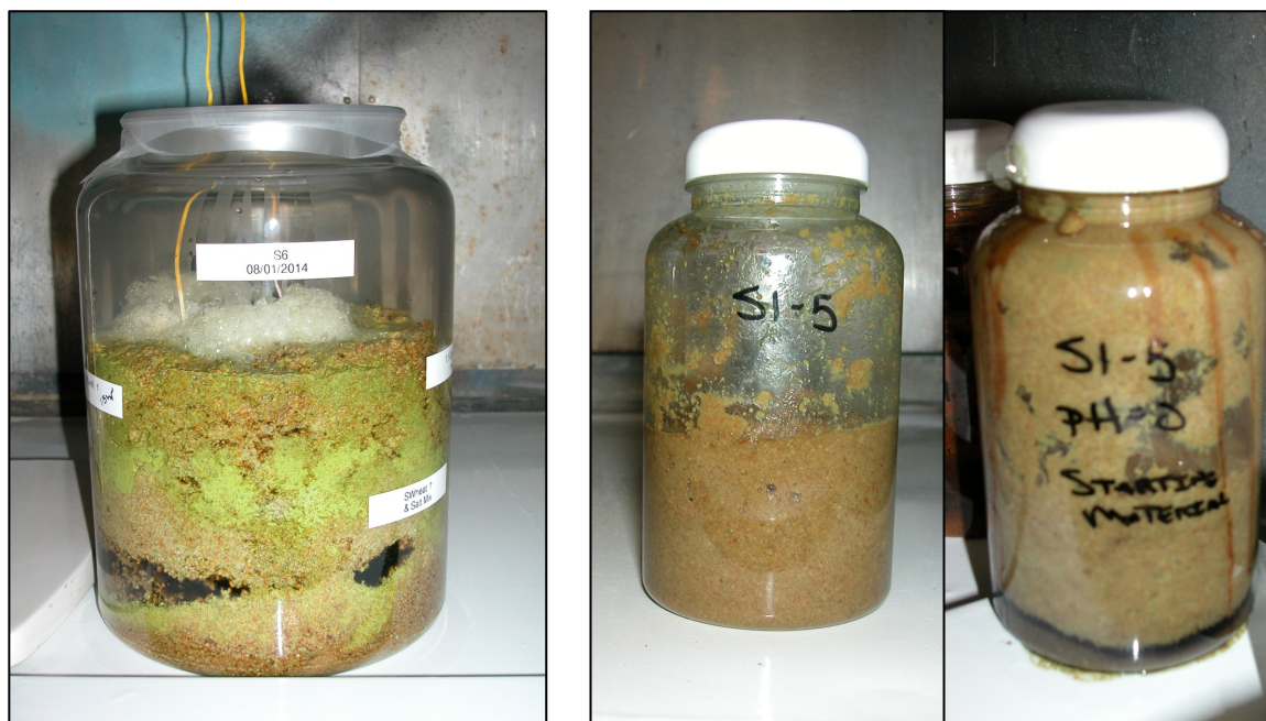
Figure 5. (left) A 3:1 (volume to volume) Swheat to nitrate salt simulant ratio containing oxalate, that was ‘quenched’ using tap water at a 1:1 (mass to mass) ratio based on mass of Swheat in sample. There is clear bubble formation as evidence of gas generation on the surface of the sample. (right) Sample S1-5 is a simulant sample prepared on 23 June 2014. A 3:1 (volume to volume) Swheat to nitrate salt simulant ratio, that was ‘quenched’ using tap water at a 1:1 (mass to mass) ratio based on mass of Swheat in sample. Sample sat relatively undisturbed since mid-July, albeit with occasional handling, but no evidence of pressurization or unusual visual characteristics. Approximately 50 days later, a Leak/burp was noticed on 12 August 2014.
