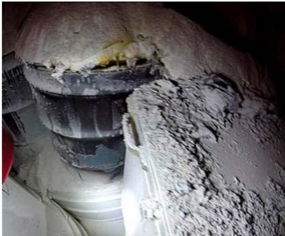
**Figure 1.6 Photo of ruptured drum in room 7, panel 7 at WIPP**
