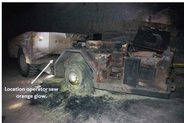
**Figure 1.4 EIMCO Haul Truck 74-U-006B after Fire**
