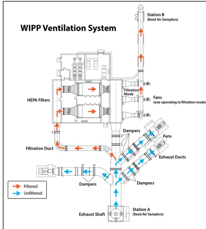
Figure 2.3 Overview of WIPP Ventilation System
