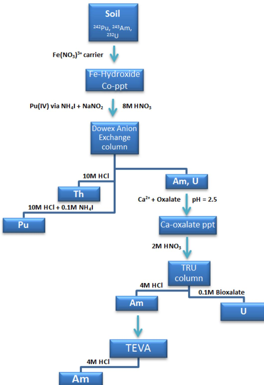
Figure 4.3 Radiochemical separation of Soil Samples
