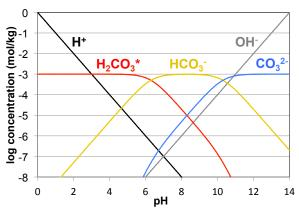
Distribution of aqueous species in the carbonate system with a total carbon concentration of  $10^{-3}$  mol/kg.
