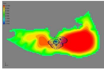
Simulated heads due to municipal well field pumping and wellhead delineation zone for Nantucket Island, Massachusetts using MODFLOW-GMS.
