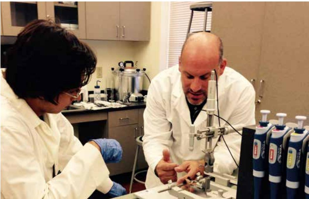
Dr. Thompson explains the robot stereotaxic, which is used to drill holes in the skull of a mouse: electrodes placed in the holes can be used to record brain waves, and examine stages of sleep.
