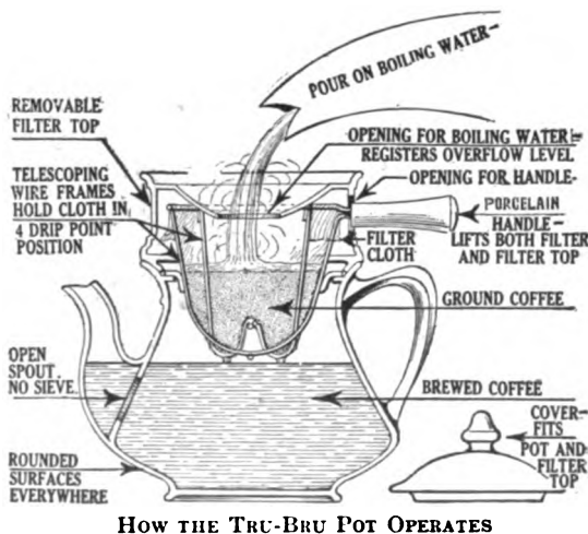
HOW THE TRU-BRU POT OPERATES
