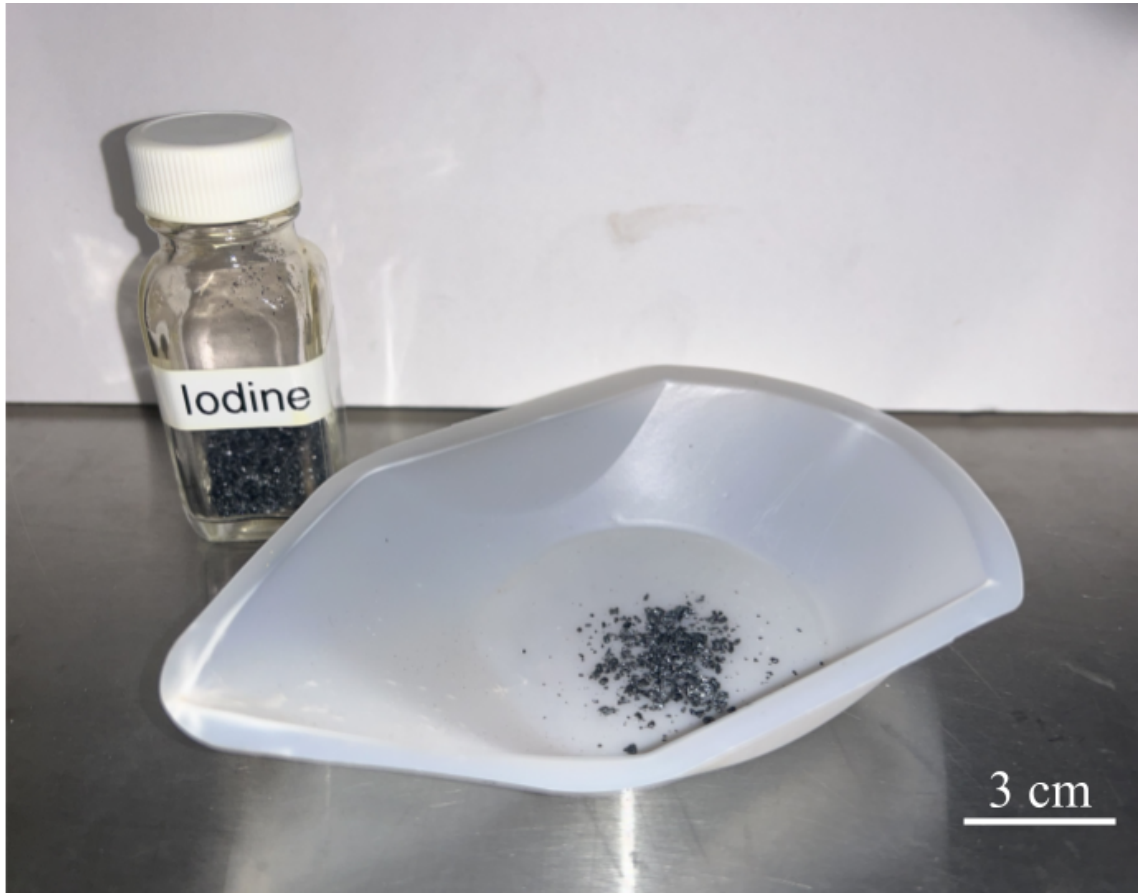
Figure 2.9: Solid iodine grains used in experimental testing.
