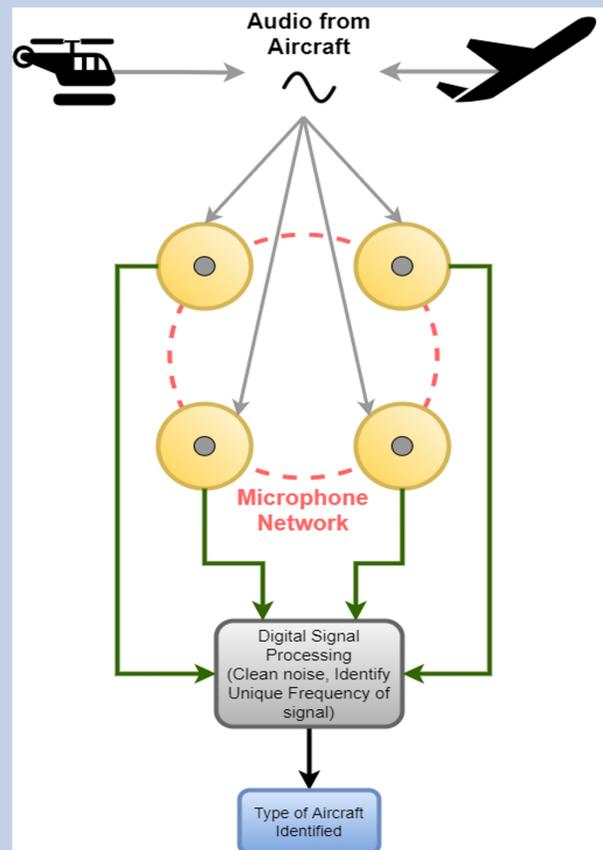
Figure(1): Working Principle of Design
