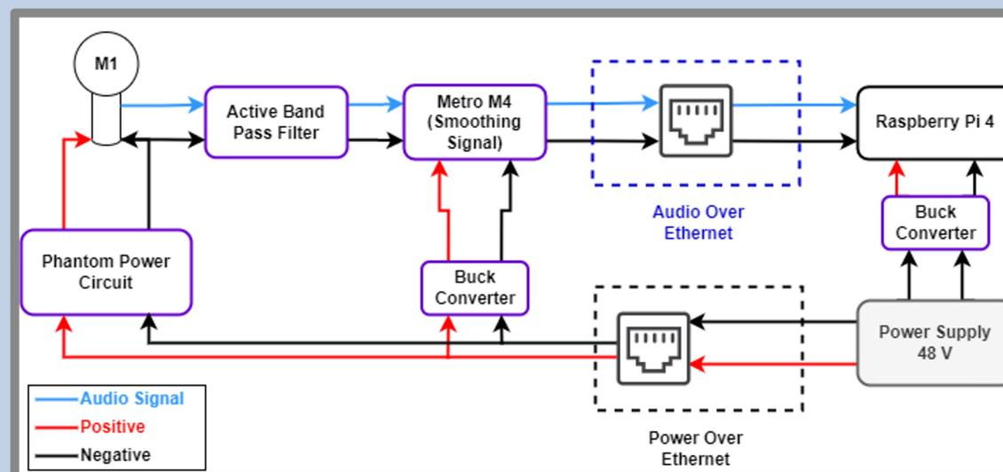
Figure(3): Final system model of single channel
